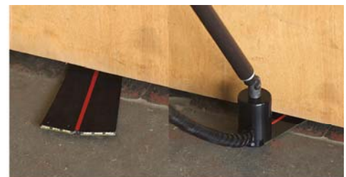
The probe will fit under most doors with it's .157" height and 2" width.
